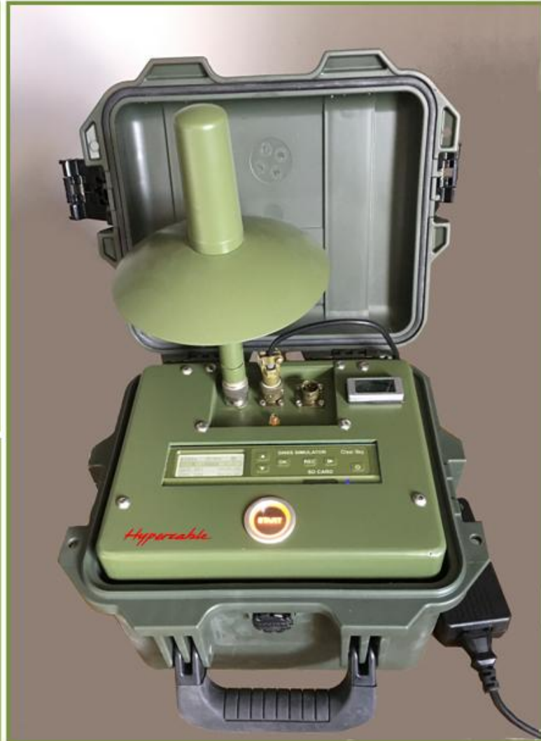
IDU GNSS simulator, power supply, amplifiers & antenna
